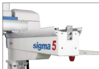
Traverse Frame Structure
